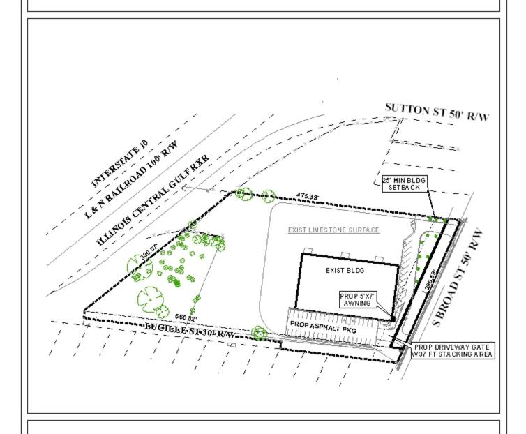
The site plan illustrates the proposed awning and vehicle stacking area.
