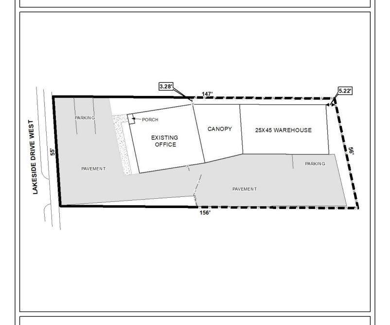
The site plan illustrates the existing building, new warehouse, and parking and manuevering area.
