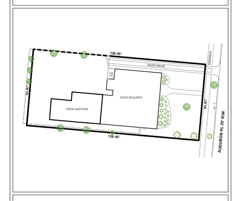
The site plan illustrates the existing building, existing drive, and proposed addition.
