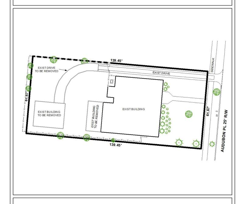
The site plan illustrates the existing building, existing drive, drive to be removed, and building to be removed.
