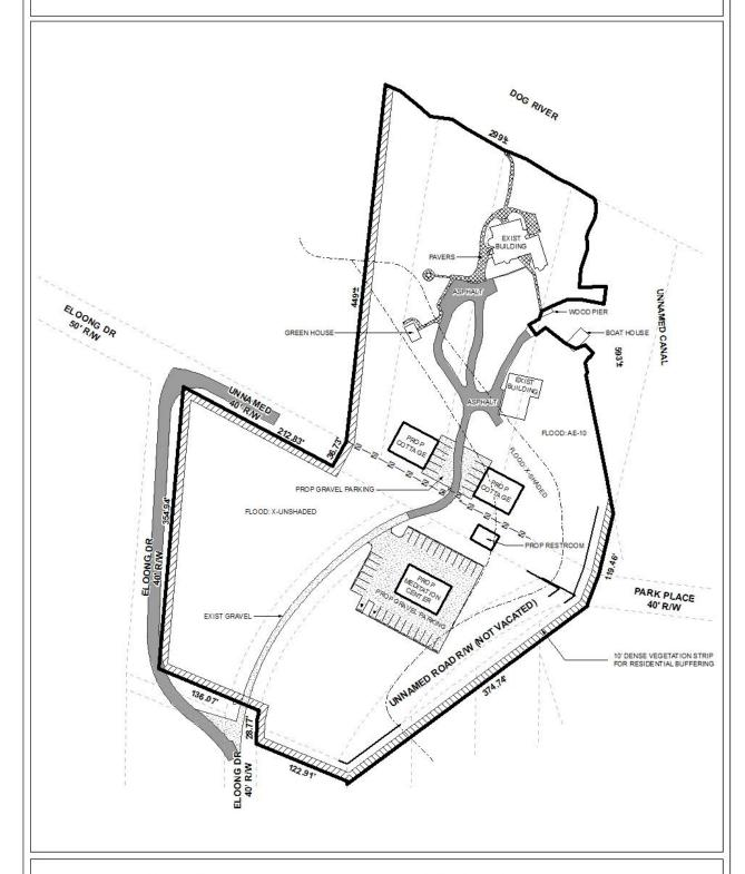
The site plan illustrates the existing gravel and asphalt drives, existing buildings, proposed gravel parking facilities, proposed buildings, and proposed vegetation strip.
