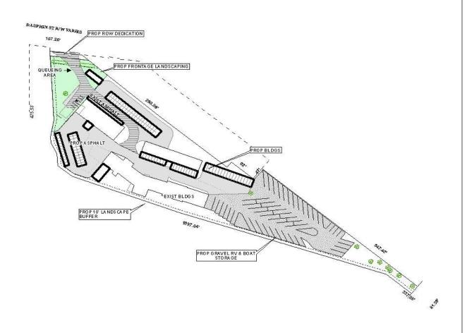
The site plan illustrates the existing structures, proposed structures, and proposed RV and boat storage area.
