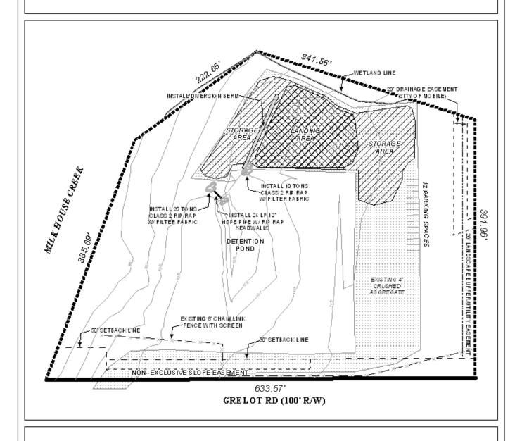
This site plan illustrates the proposed material/equipment storage yards and helicopter landing area.
