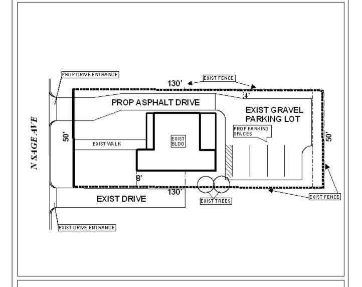
The site plan illustrates the existing building, drive, landscaping, and parking area along with the proposed asphalt drive, entrance, and parking configuration
