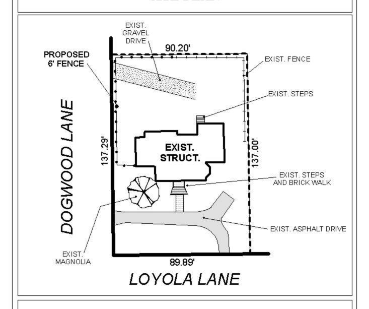
The site is located at the Northeast corner of Loyola Lane and Dogwood Lane. The plan illustrates the existing structure and the proposed fence.
