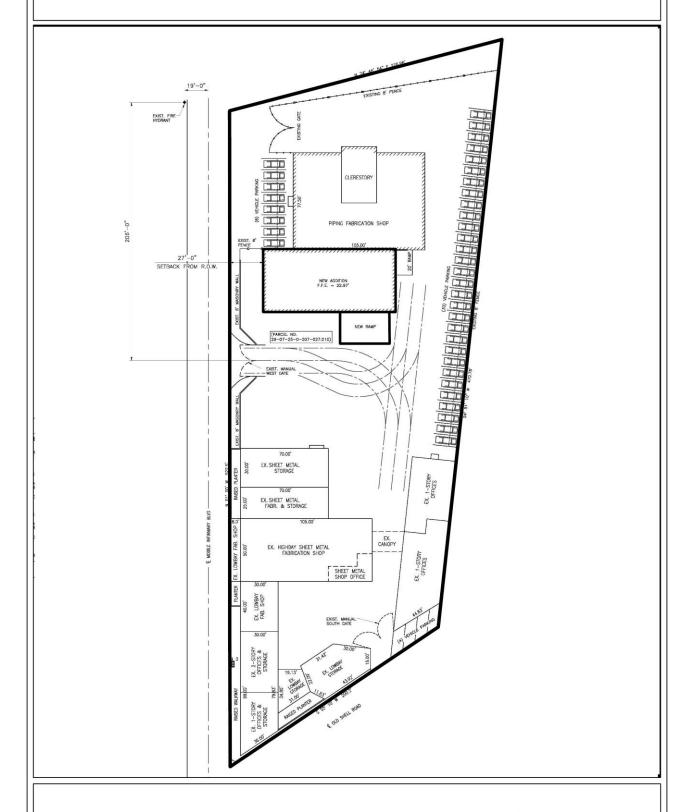
The site plan illustrates the existing buildings, parking, proposed addition, and proposed ramp.
