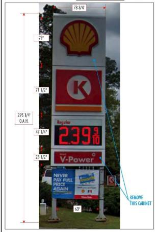
PROPOSED LEDS SIZES: REUSE 24" RED ABLE 7-SEG. LEDS NEW 24" GREEN ABLE 7-SEG. LEDS
