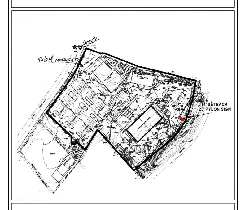
The site plan illustrates the existing building, and pylon sign location.
