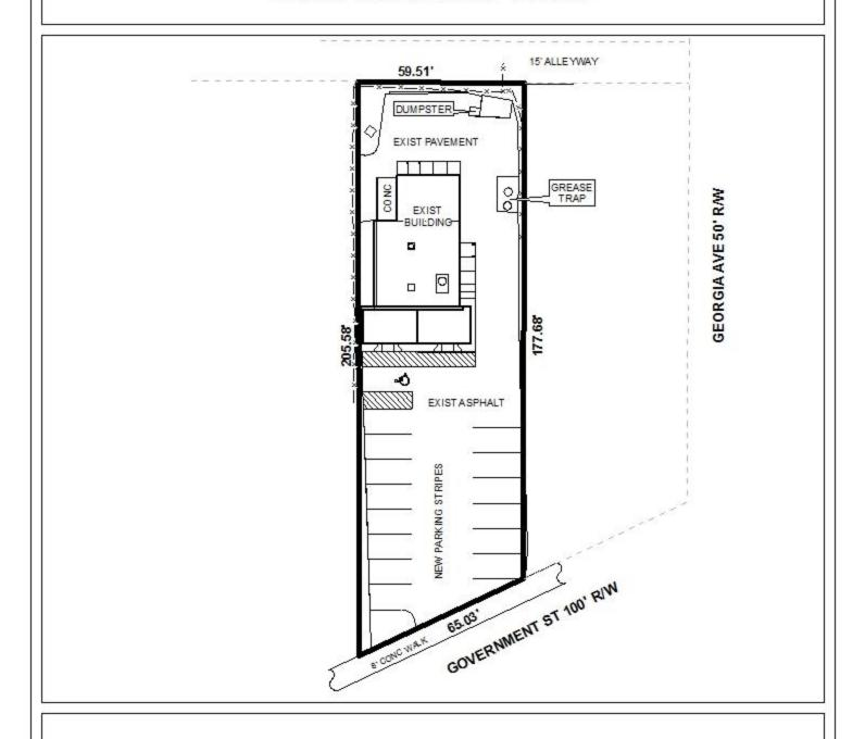
The site plan illustrates the new parking additions, existing building, and fence.
