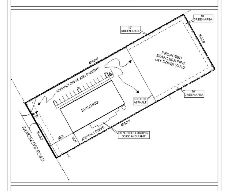
The building, parking, drive, and proposed pipe lay down yard are illustrated in the site plan.
