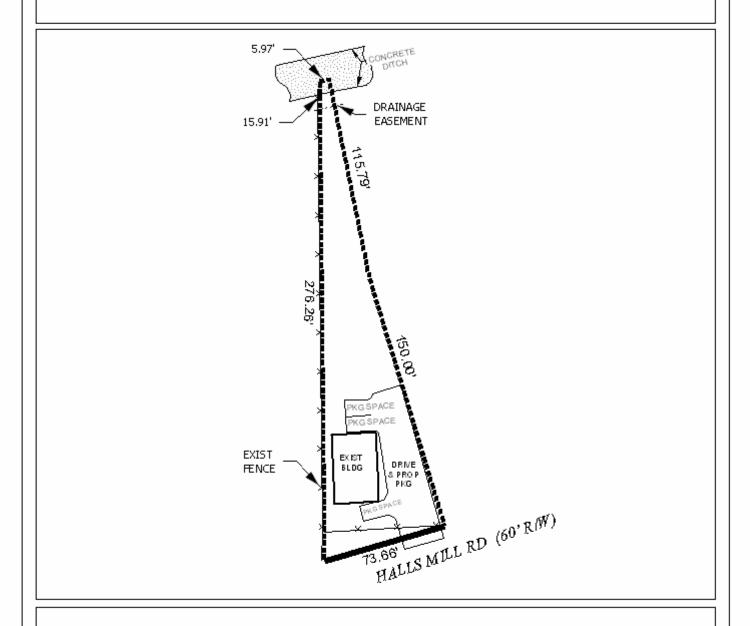
The site plan illustrates the existing building, fence, proposed parking, and drainage easement at property rear.
