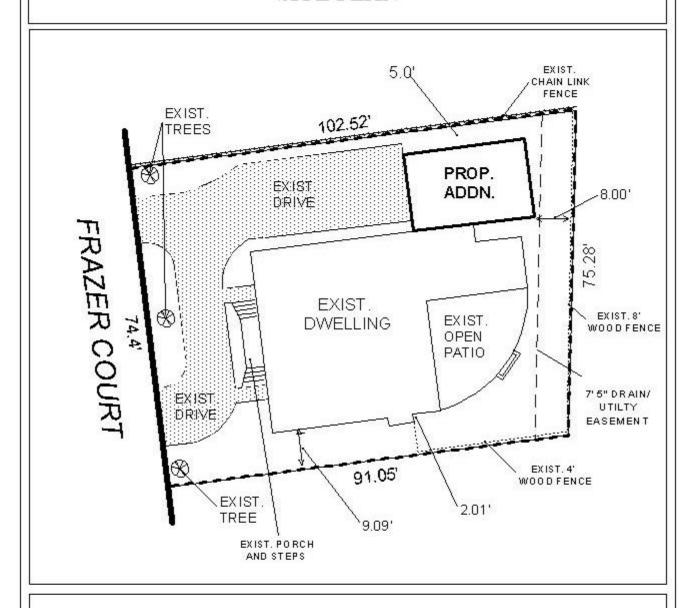
The site is located on the East side of Frazer Court, 279' North of Old Shell Road. The plan illustrates the existing and proposed structures.
