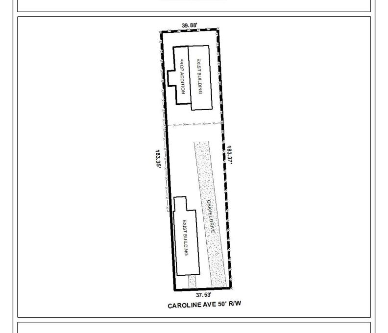
The site plan illustrates the existing buildings, gravel drive, and proposed addition.
