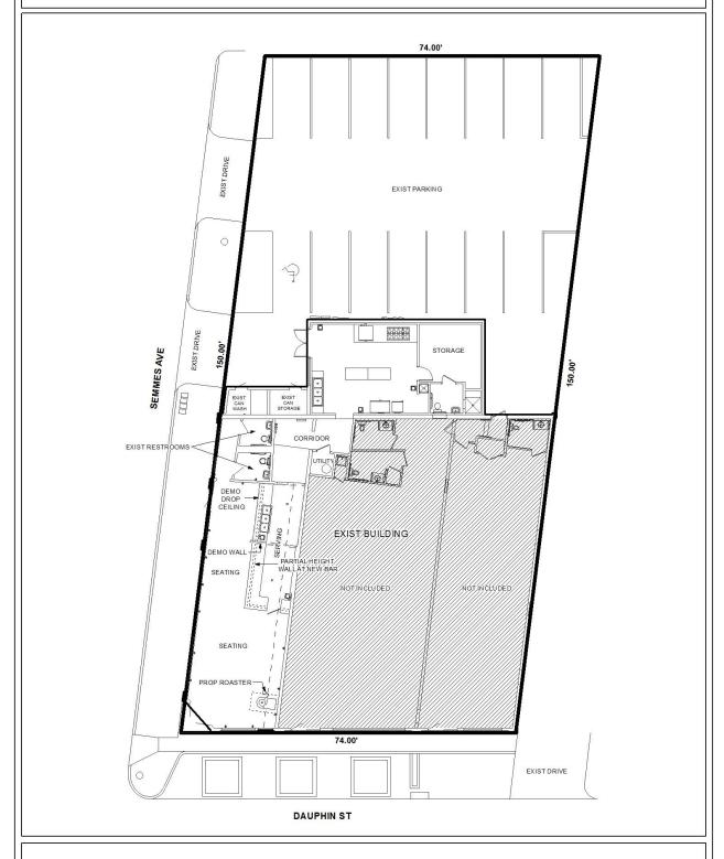
The site plan illustrates the existing building, existing parking, existing drive, walls to be demoed, and proposed layout additions.
