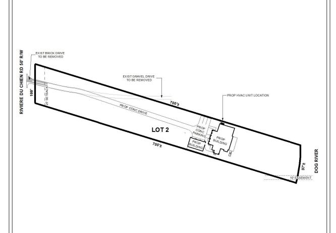
The site plan illustrates the proposed drive, proposed buildings, proposed HVAC unit location, setback, and easements.
