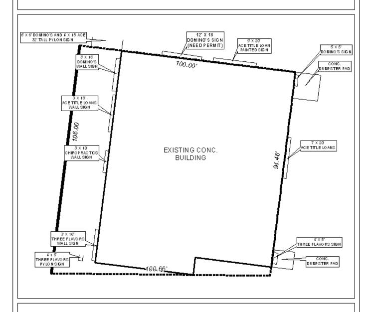
This site plan illustrates the existing building and sign locations. The proposed Domino's sign is located on the north side of building.
