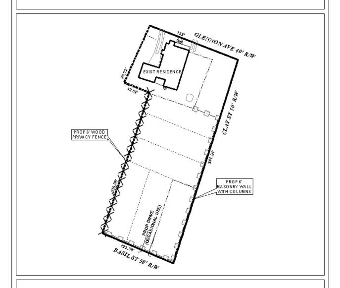
The site plan illustrates the proposed wood fencing and masonry wall.
