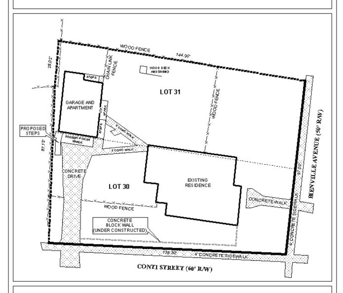
This site plan illustrates the existing structures and lot configuration. A concrete block wall is under construction on the south boundary. The proposed steps are located at the southwest corner of the garage and apartment.
