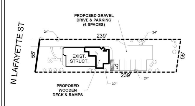
The site plan illustrates the existing buildings, proposed building addition, and proposed parking.
