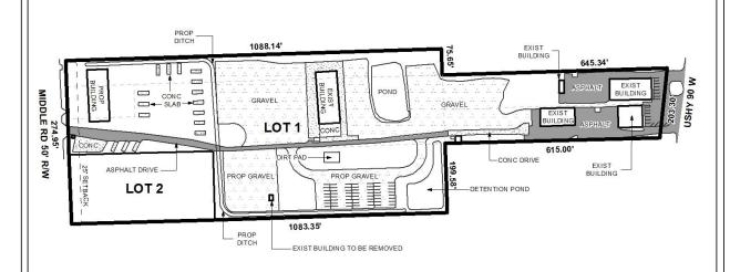
The site plan illustrates the existing buildings, existing drive, setback, proposed building, proposed gravel areas, and proposed ditch.
