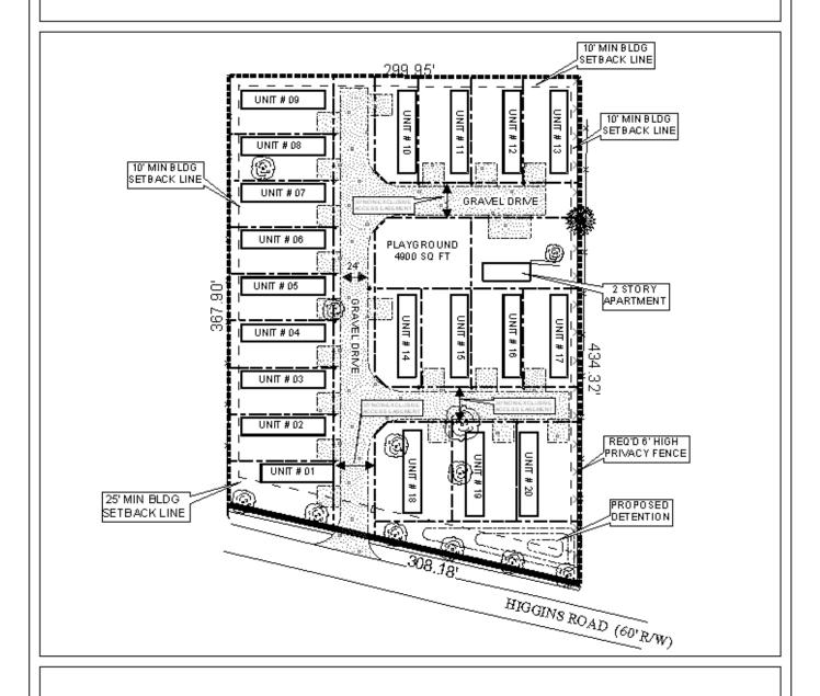
The site plan illustrates the lot configuration, drives, access easements, setbacks and location of structures.
