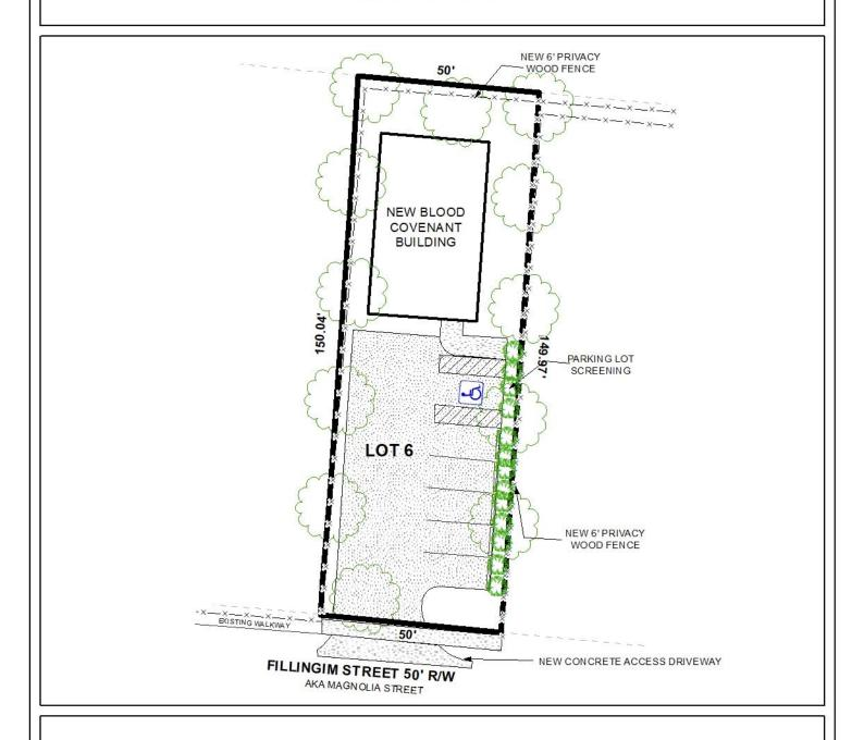
The site plan illustrates the proposed building, fencing, concrete access, and parking area.
