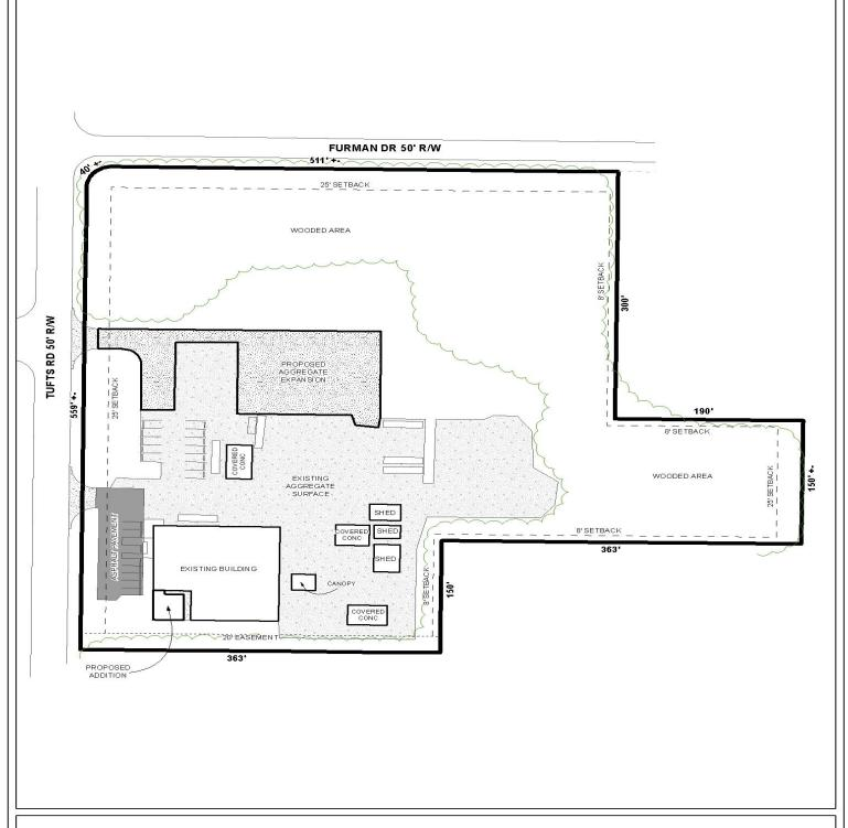
The site plan illustrates the proposed building addition, the proposed aggregate expansion, setbacks and easements.
