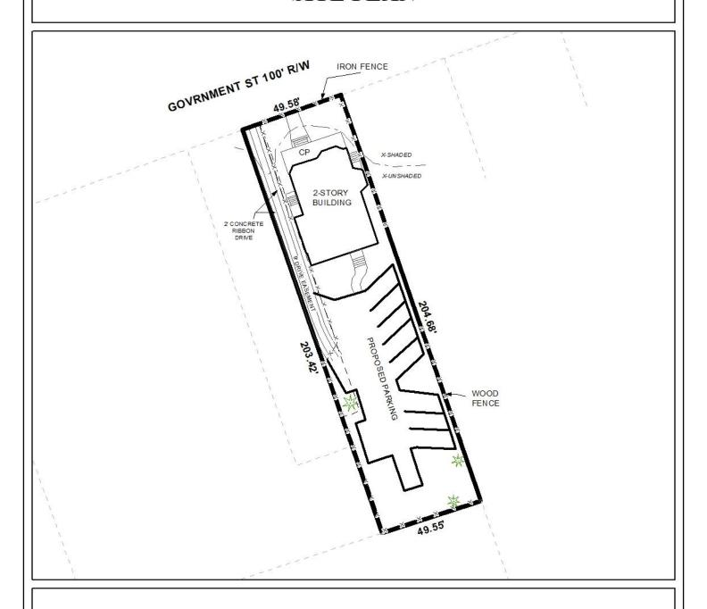
The site plan illustrates the existing building, drive, easement, and proposed parking.
