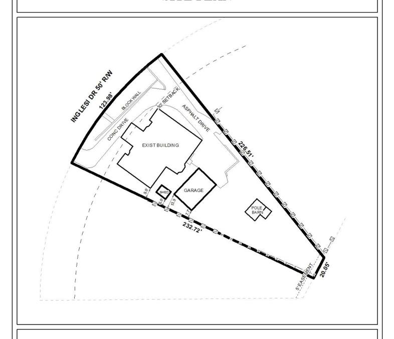
The site plan illustrates the existing building, proposed garage and shed, setback, and easement.
