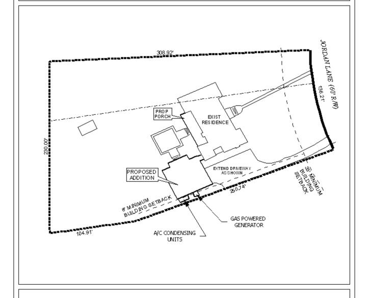
Illustrated in the site plan are the proposed A/C condensing units, the gas powered generator, addition and setbacks.
