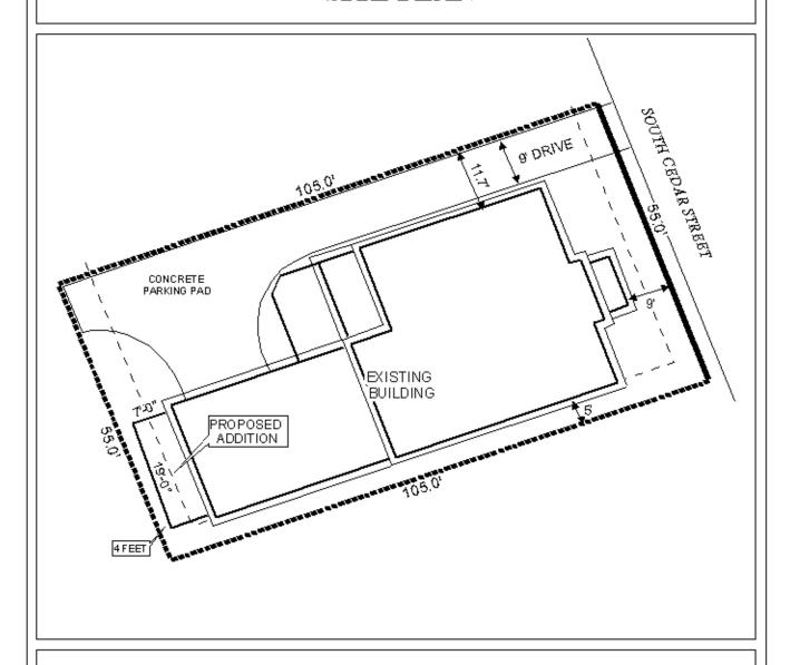
Drive, parking, existing and proposed structures are represented in the site plan.
