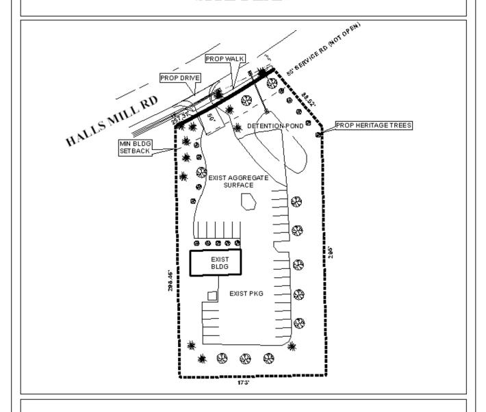
The site plan illustrates the existing building, parking, aggregate surface area, proposed landscaping, and detention area
