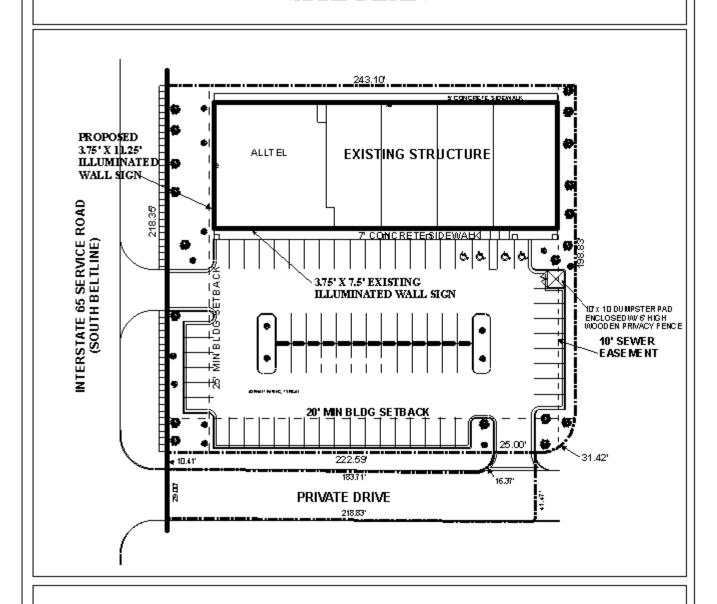
The site is located on the East side of Interstate 65 Service Road South, 700' South of Emogene Street. The plan illustrates the existing structure and parking.
