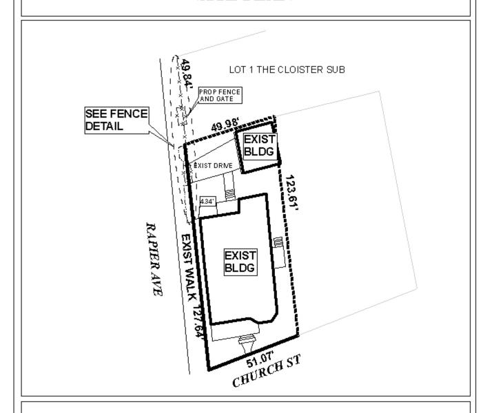
The site plan illustrates the existing buildings and drives along with the proposed fencing and setbacks.
