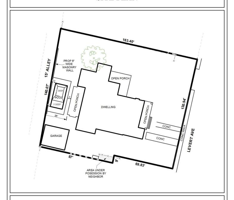
The site plan illustrates the existing dwelling, proposed pool, and masonry wall.
