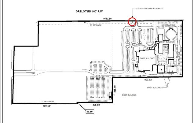
The site plan illustrates the existing buildings, easements, setbacks, and sign to be replaced.
