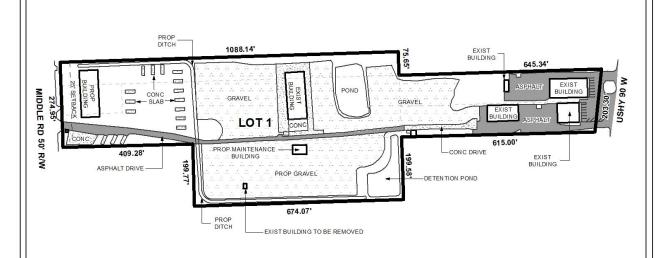
The site plan illustrates the existing buildings, existing drive, setback, proposed buildings, proposed gravel area, and proposed ditch.
