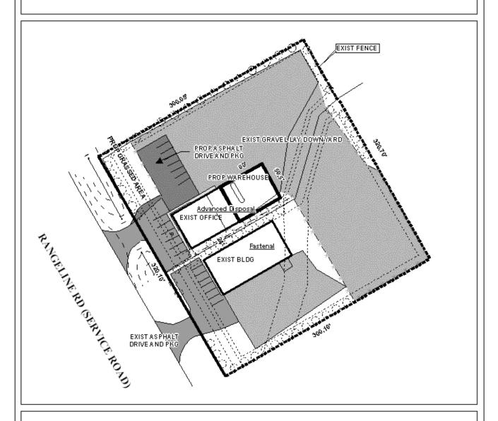
The site plan illustrates the existing building, gravel laydown yard, proposed asphalt drive, proposed asphalt parking, and the proposed building addition.
