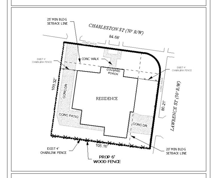
The site plan illustrates the existing residence, concrete walks, drives, patio, existing chainlink fence, and proposed wood fence.
