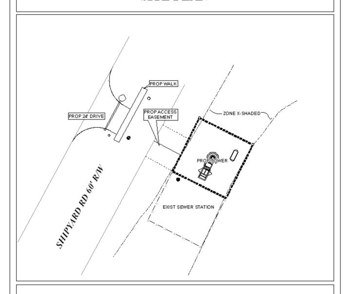
The site plan illustrates the proposed tower location, access easement, drive and walk
