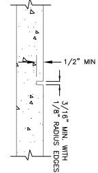
CONTROL JOINT DETAIL NOT TO SCALE
