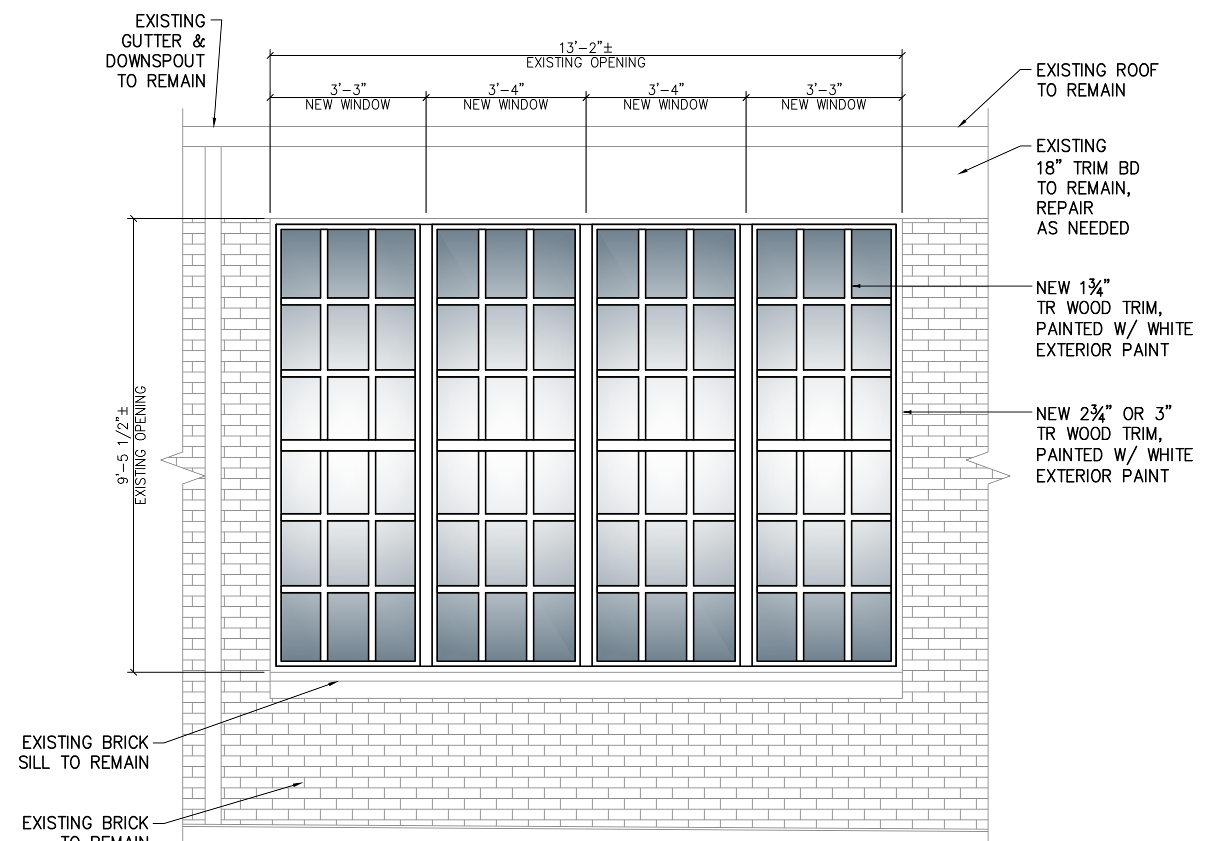
WEST WINDOW TRIM ELEVATION SCALE: 1/8"=1'-0"
